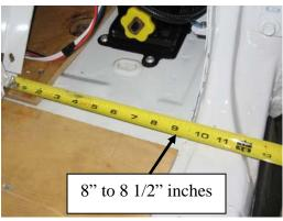
Measurement from passenger-side **Rear Doorframe** to vehicle doorframe shown above
